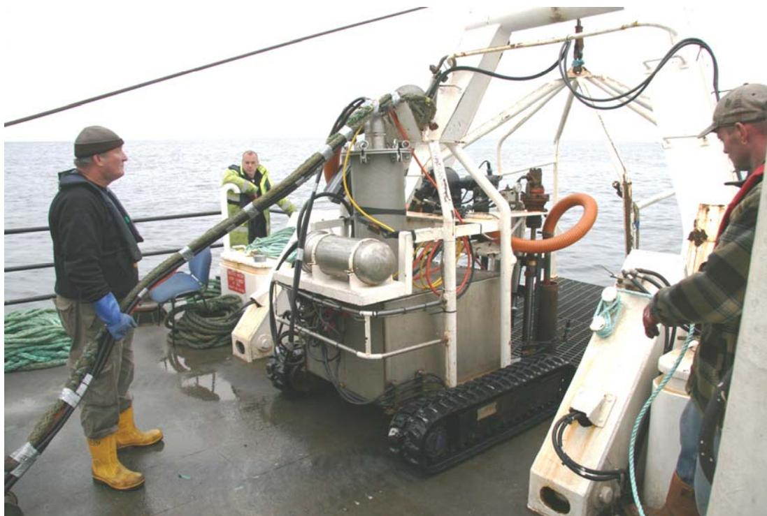
Figure 4. The modified ROV used for offshore cleanup trials in August and September 2008.
